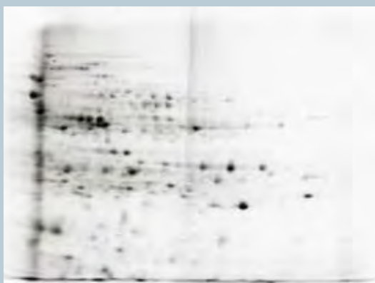
2D electrophoresis on SERVAGe™ TG PRIME™ 14 % vertical mini gel stained with SERVA HPE™ Lightning Red
