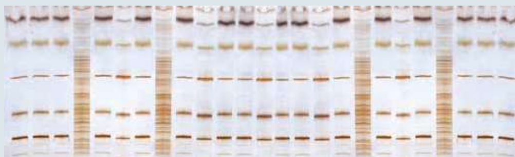
Proteins ( E. coli lysate, protein standards) separated on 12.5 % 1D SDS Excellent gel.
